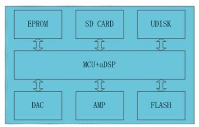
Module selection is the SOC program, integrated a 16 -bit MCU , and a dedicated audio decoding aDSP , the use of hard decoding, more to ensure the stability of the system and sound quality. Small package size to meet the needs of other products embedded
